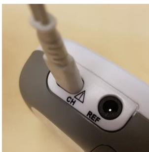
3. Cross over the metal pins at the end of the electrode lead and firmly hold them together, thereby creating a circuit
